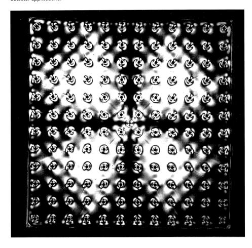
type of sampling calorimeter with wavelength-shifting fibre readout developed recently by IHEP with INR (Moscow), where "perforated" scintillator tiles (see cover photograph, April 1993) with many precision-positioned holes.
