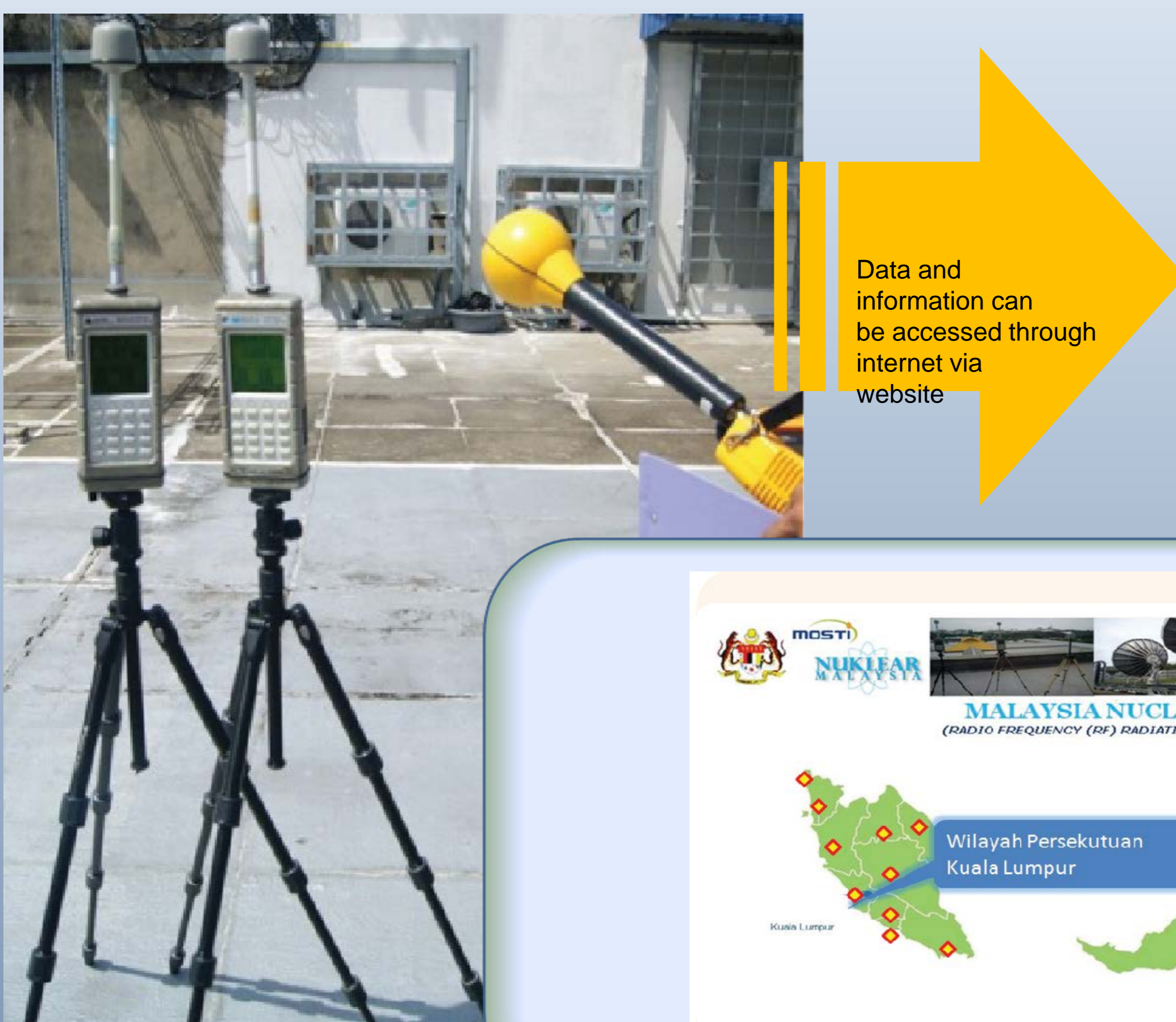
Figure 8: Equipment for RF assessment and data acquisition process
