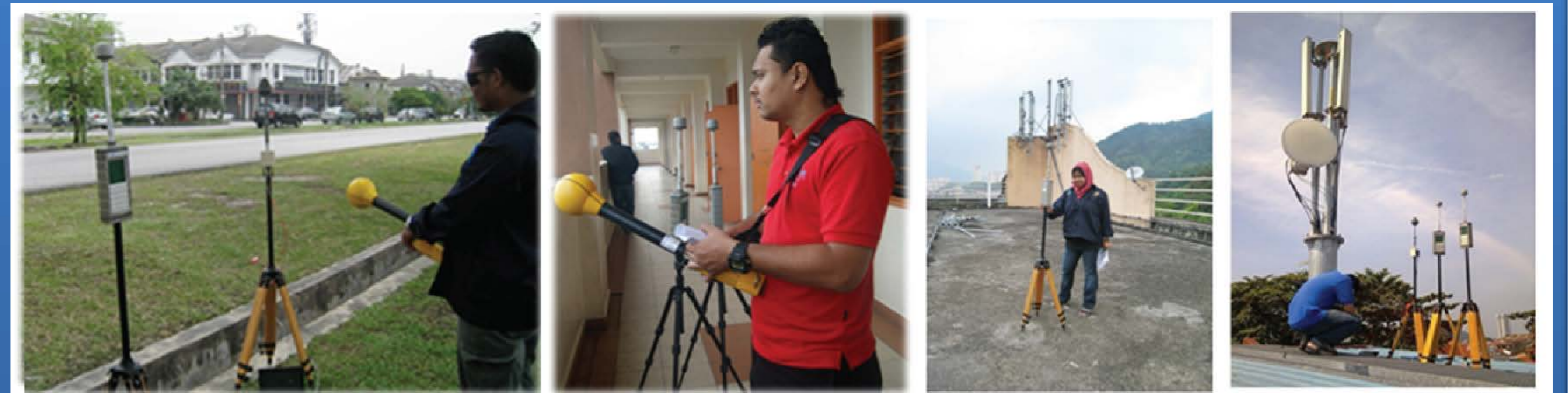
Figure 4: RF radiation assessment around telecommunication structure adjacent to residential area and school
