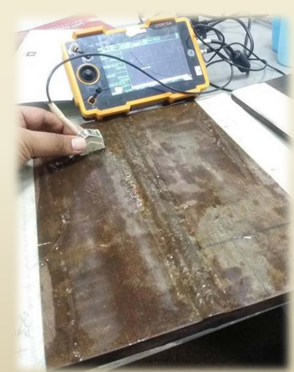
Inspection using Conventional Ultrasonic
