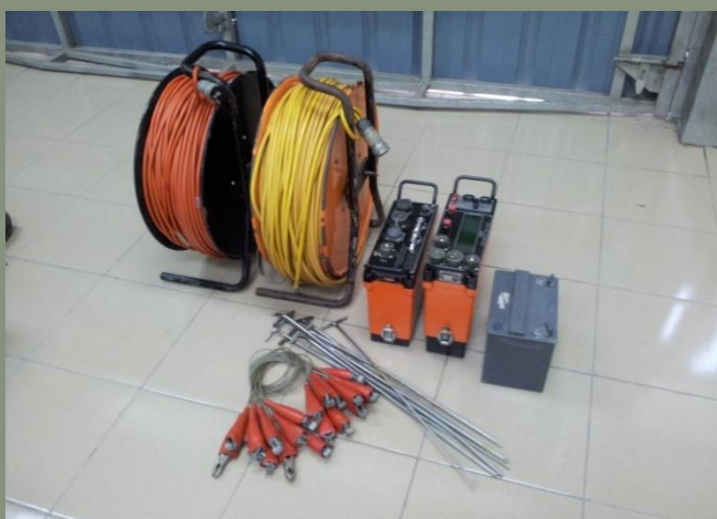
Figure 1: ABEM Terrameter SAS4000, electrode selector, multicore cables, clips, electrodes and battery
