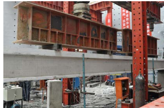
Fig.3 Loading scheme and test instrumentation.
