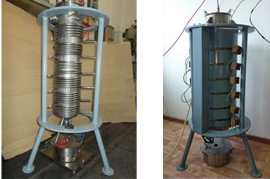
Fig. 4 - Experimental facility: intermediate stage - without insulation (left)/ with insulation (right)
