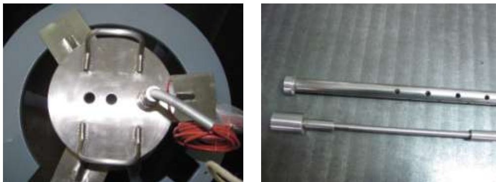
Fig.3 Removable circular cover – top view (left); reflector and support tube (right)
