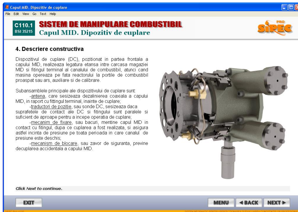
Fig.4 – F/M Head Coupling device
