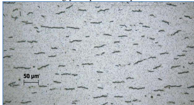
Fig 1. Micrograph showing hydrides in Zr-2.5%Nb pressure tube
