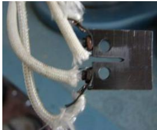
Fig.6 The CT specimen wired for PD method
