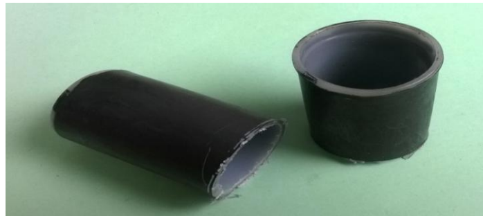
Fig. 8. Graphite deposition on polyethylene layer [6]
