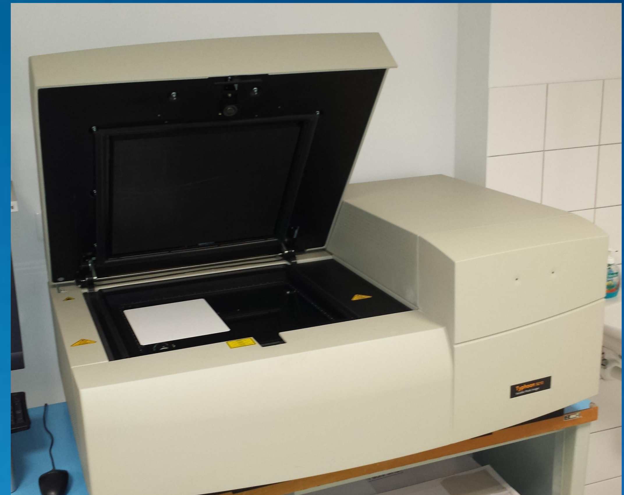
obr. č. 1: Image scanner Typhoon 9210 s pamäťovou fóliou storage phosphor screen BAS-MS 2025
