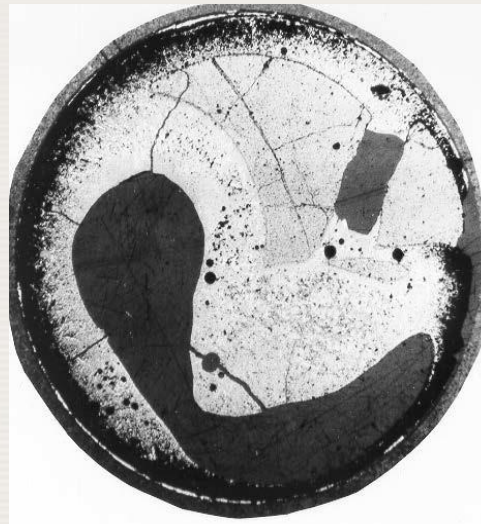
ITU SETs: Fresh fuel rod segment: Dissolution at 2000° C / 190s
