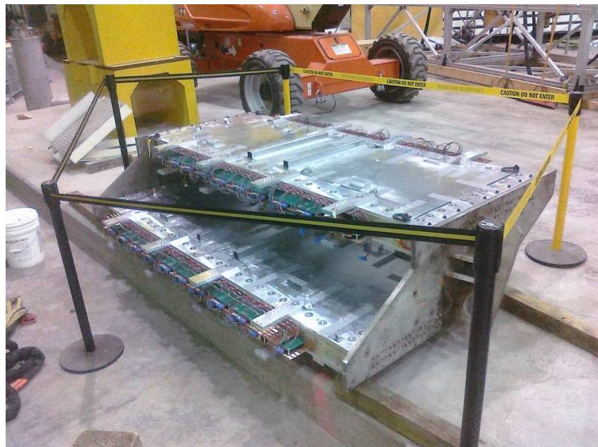
Figure 4. One of two pairs of wire chambers on loan to us from the College of William and Mary for use in the Bethe-Heitler measurement.
