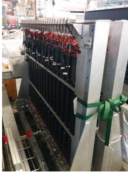
Figure 5. Trigger scintillators on loan from Tohoku University to be used in the Bethe-Heitler measurements at HI \gamma S. They were previously used at JLAB.
