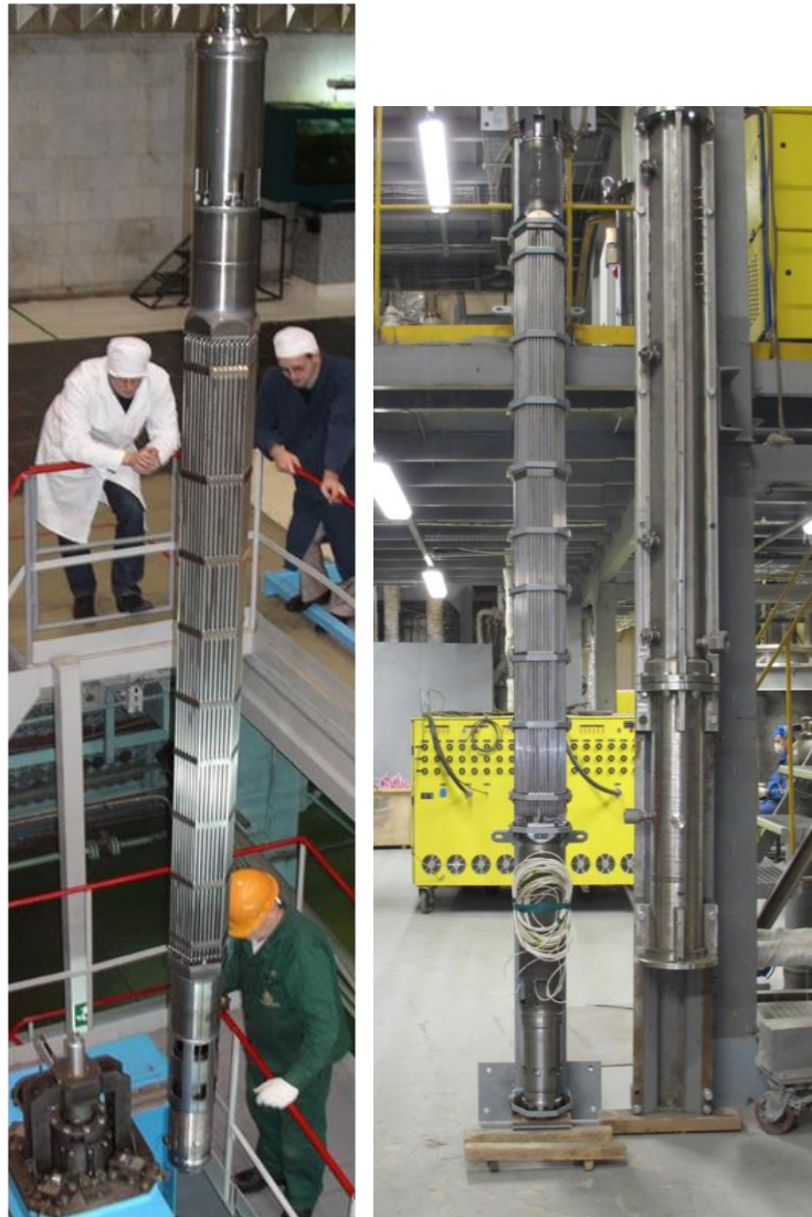
FIG. 1. Full-scale FA mock-up and FA mock-up with a retort for testing.
