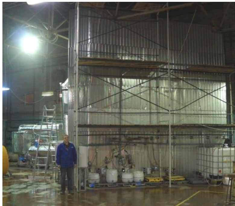
FIG. 4. Full-scale mockup of reactor vessel's central part.
