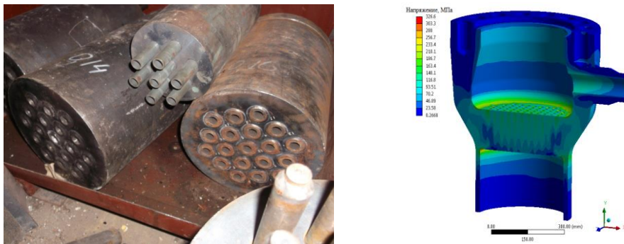
FIG. 9. Study in thermal cyclic strength of “tube-tube sheet” joint.
