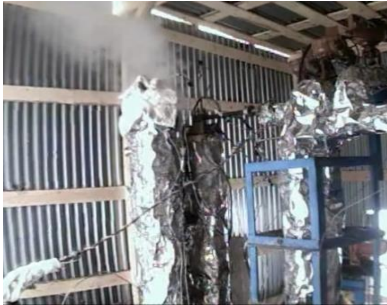
FIG. 8. Tube rupture experiment.
