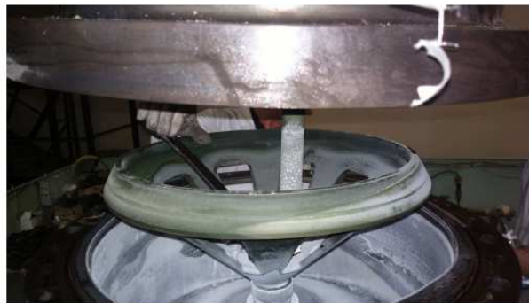
FIG. 6 – Segment of the locking element after testing.
