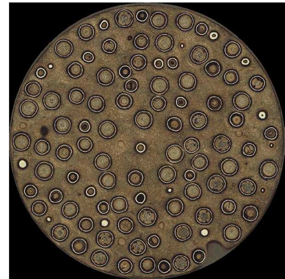
Cross section of an AGR-2 UCO fuel compact irradiated (11.0% FIMA, time-peak T 1305°C)
