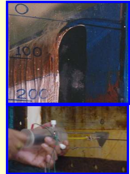
Gas entrainment at 300 mm fall height
