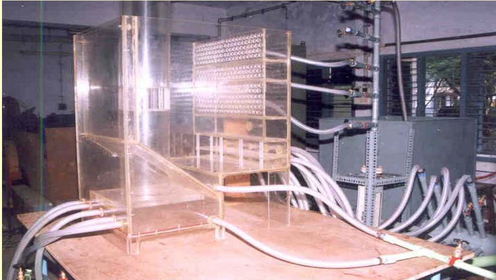
Basic studies to understand the Mechanisms responsible for GE in hot pool (1:27, 1:18 & 1:9 models)
