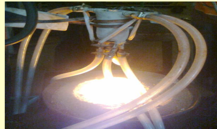
Melting of U fuel pins in ceramic crucible by induction heating
