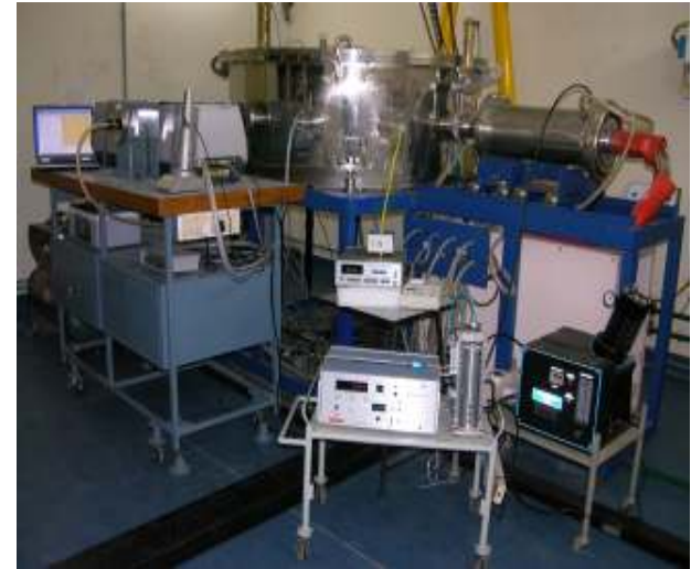
Real Time Measurements: Mastersizer, QCM , Aerosol spectrometer, ELP impactor, SMPS. OFF-Line Measurements: Filter paper tech.. Chemical analysis, Conductivity probe,etc.
