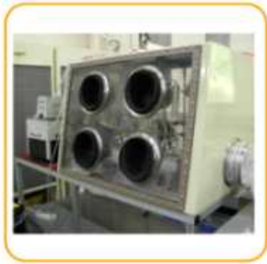
Alpha, Beta Shielded Glove Box(II)
