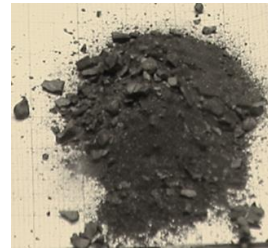
Dispersed fuel fragments from one of the NRC tests
