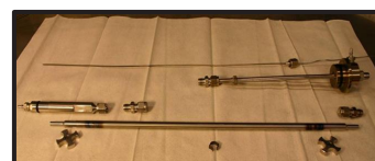
Fig 1. Front view of the LOCA apparatus showing the main parts. The total height of the apparatus is 1145 mm.
