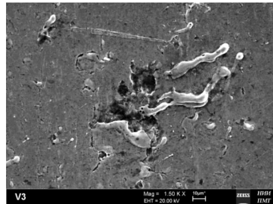
Fig. 5. The ejection of pieces (surface fragments) of an arbitrary shape in a sample irradiated with four pulses at q = 10^7 - 10^8 \text{ W/cm}^2
