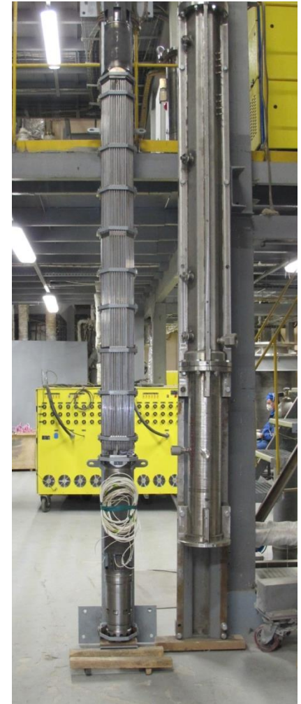
FA mock-up with a retort for testing
