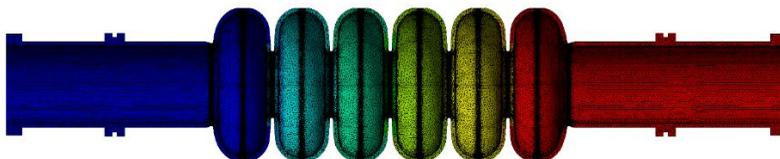
Fig. 2. SRF Cavity deformation under applied load, extra-scaled
