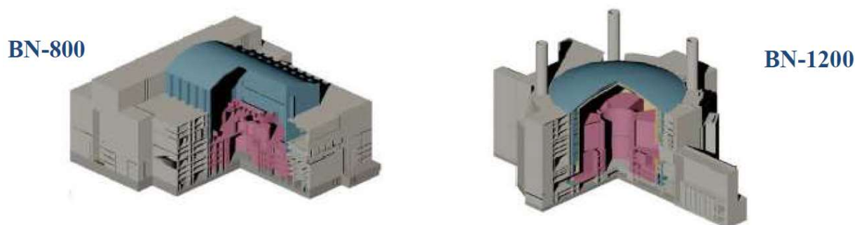
FIG. 3. BN-800 and BN-1200 reactor building schemes [20].
