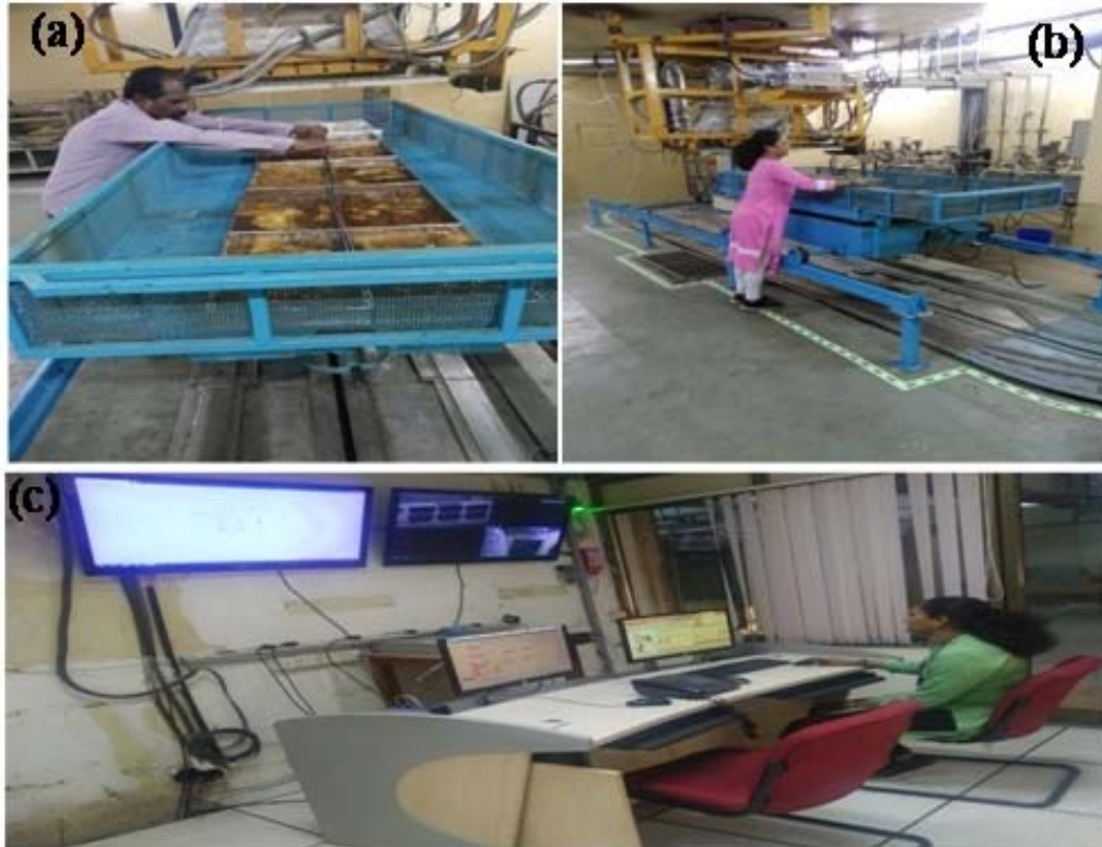
Fig.2. (a) & (b) Placement of chitosan sample on to & fro conveyor system, (c) 10 MeV Linac control room
