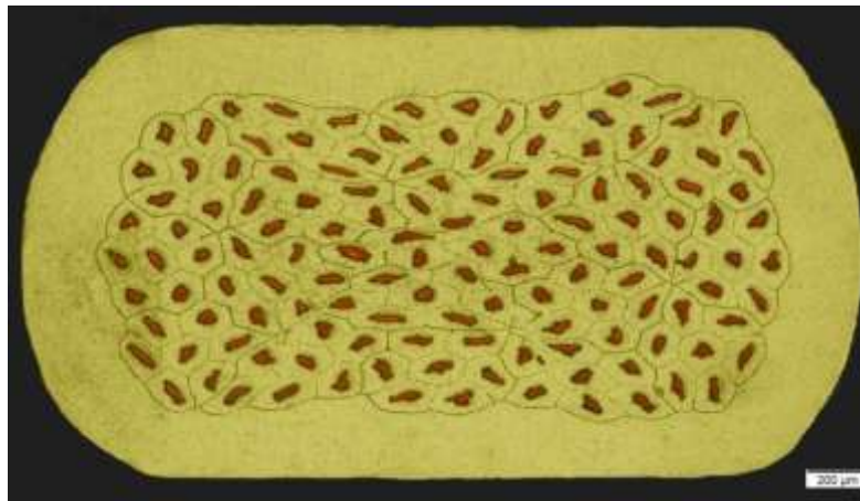
Figure 1.- Cross-section of the LEU fuel element.
