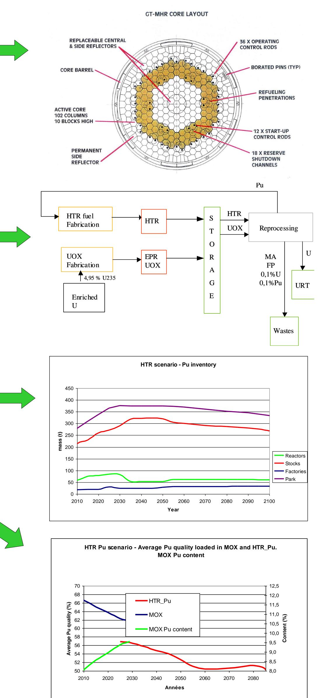
3 - The calculation of the scenario have been performed with the code COSI. This code simulates a pool of nuclear electricity generating plants with its associated fuel cycle facilities. In COSI, the CESAR code is used for the in-pile calculations. CESAR uses cross sections generated after neutronic calculations performed with the APOLLO2 code
