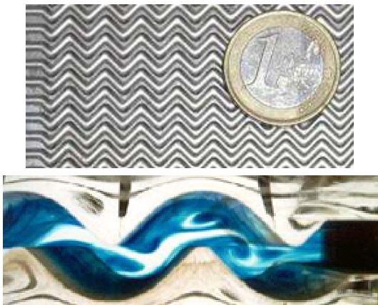
Figure 4 - Mini corrugated channels (with the courtesy of HEATRIC company).
