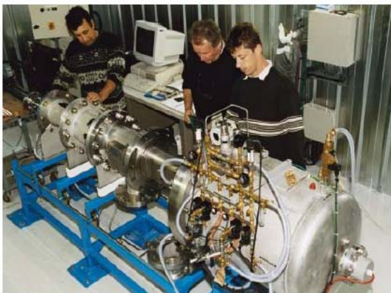
Figure 1a: View of CEA He tribometer
