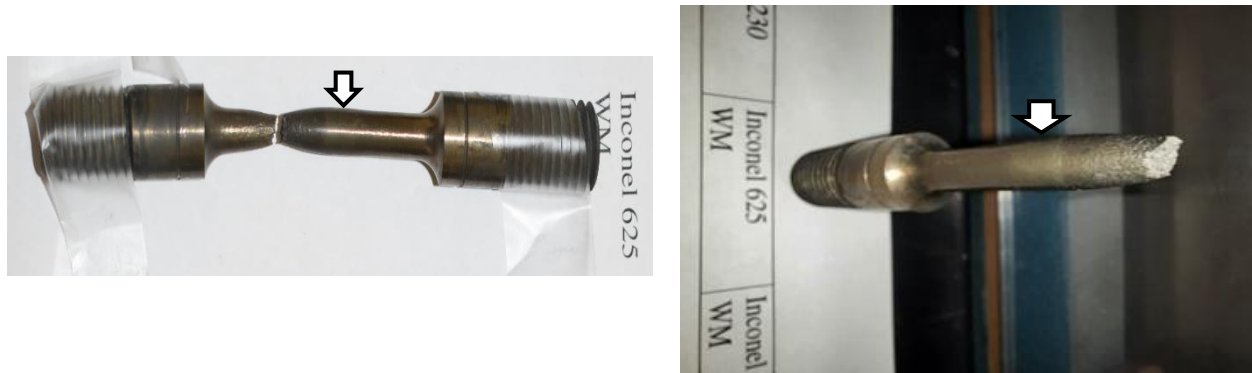
Figure 6: Typical Fracture Mode of Incoloy 800H Welds with Inconel 625 Filler Material
