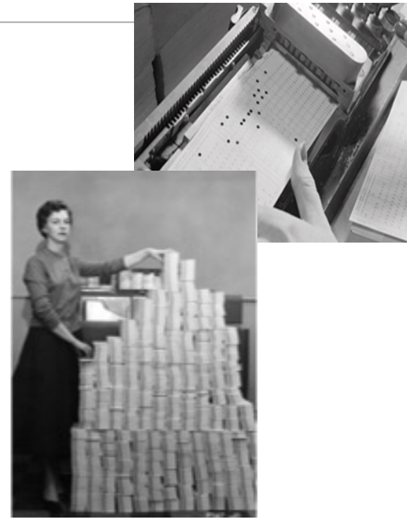
This stack of 62,500 punched cards — 5 MB worth — held the control program for the giant SAGE military computer network.
