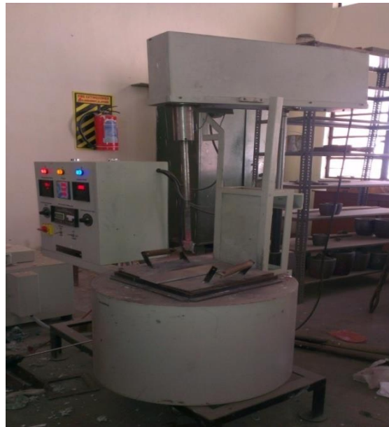
Figure 1: Aluminium stir casting setup
