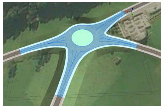
Figure 4. A roundabout is automatically added by changing the type of intersection where two or more roads are in close proximity.
