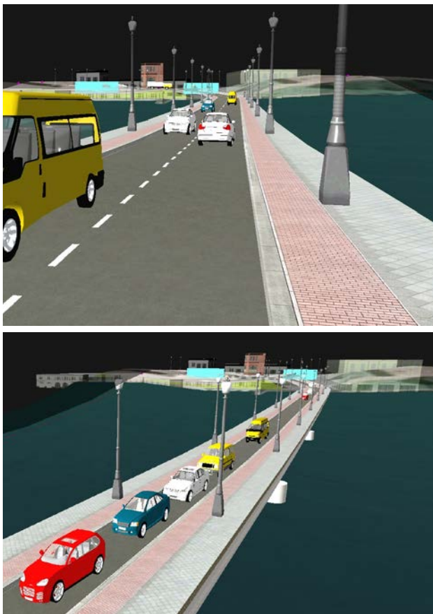
Figure 10. Some images of the simulation with 1 (bottom) and 2 lanes (top). The 3D model of the bridge is not the one generated from laser point clouds, as a detailed geometric model was not necessary for such traffic analysis. A simplified model of the bridge was generated via parametric modelling, changing in an automatic way the number of lanes.
