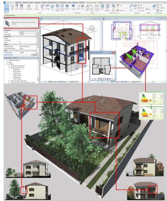
Figure 2. As-built BIM of a (simplified) building obtained with the parametric modelling logic of BIM software.
