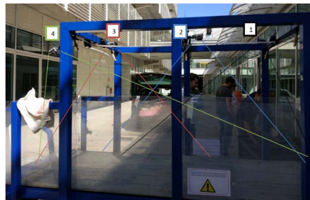
Figure 2. Locations of four GoPro 4 Black® cameras on the 'Landslide Simulator' and the field-of-view of each sensor.
