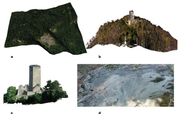
Figure 5. Digital 3D data derived from multi-scale integrated survey campaigns: (a) a sample of aerial LiDAR flight with (b) zoomed view on the Baradello tower and (c) Baradello tower from photogrammetric flight 3D model and (d) the textured LiDAR mesh particular of a carved rock in Pianvalle.
