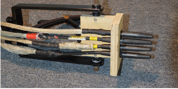
Figure 2: The constructed microphone array of M = 4 sensors.
