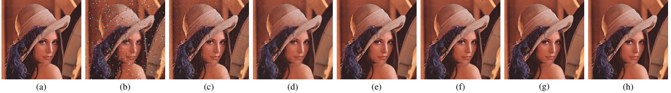
Fig. 3. Super-resolution results for the corrupted ‘Lena’ image with mixed noise ( r = 2 ). (a) Ground truth, (b) LR image (first frame), (c) L_2 + Tikhonov (PSNR:27.33,SSIM:0.91), (d) L_2 + BTM (PSNR:29.43,SSIM:0.94), (e) L_1 + BTM (PSNR:29.69,SSIM:0.94), (f) BEP (PSNR:30.77,SSIM:0.96), (g) IRWSR (PSNR:31.98,SSIM:0.97), (h) Proposed (PSNR: 33.19 ,SSIM: 0.98 ).
