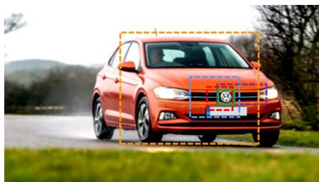
Fig. 1 Diversity of bounding box regression, where green box is the ground-truth box
