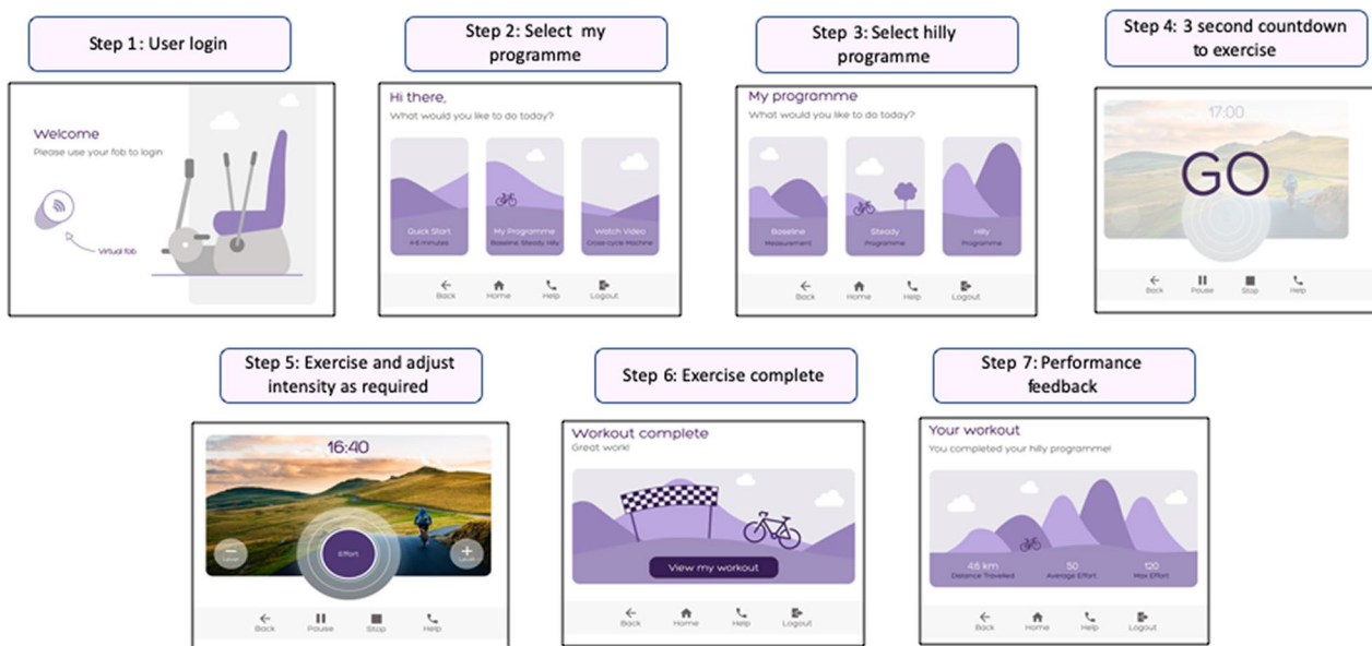
Fig. 10 Graphical User Interface Version 2 hilly exercise programme menu: The white margin outside the purple circle indicated the target effort for the user
