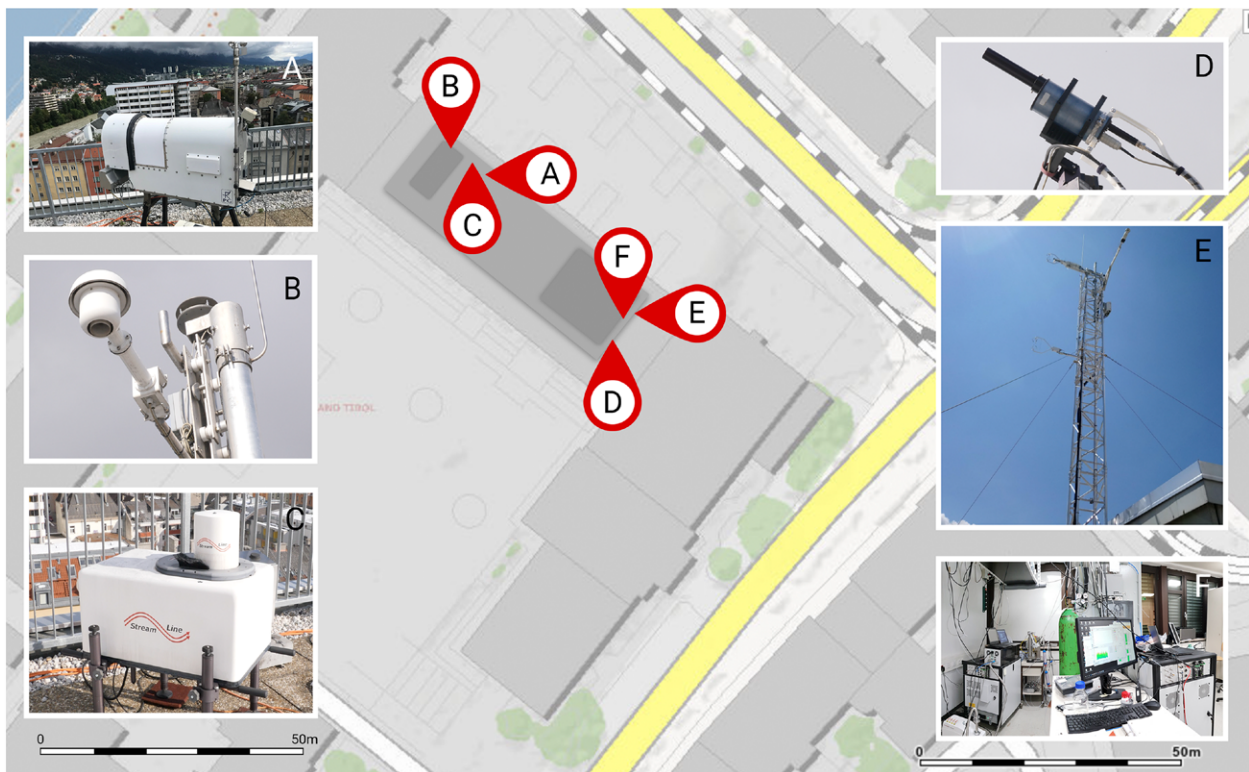
Fig. ES2. Top view of the IAO facilities: (a): microwave sounder, (b) TAWES weather station, (c) Doppler wind lidar system, (d) Pandora, (e) flux tower, and (f) laboratory facilities. Map data obtained from Land Tirol (TIRIS).
