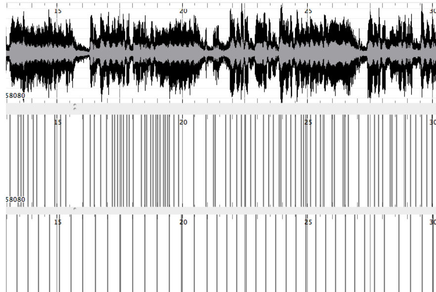
Figure 2.17: Rhythm seen as periodicity of onsets. Example for an input signal (top), with estimated onsets (middle), and estimated beat positions (bottom).
