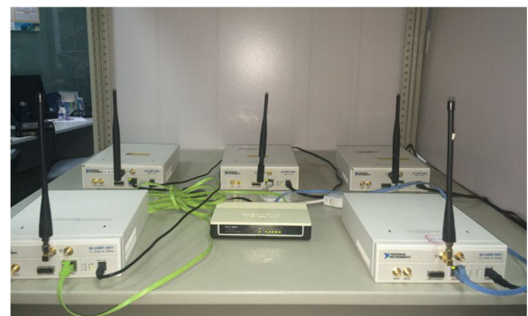
Fig. 8 SDR platform implemented by USRPs
