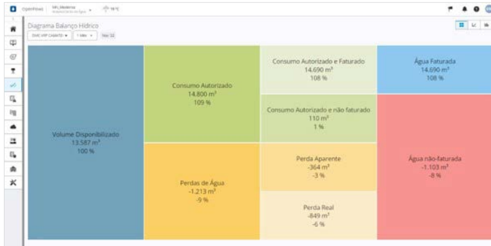
Figure 4: Water balance reported with consumption billed volume greater than distributed.
