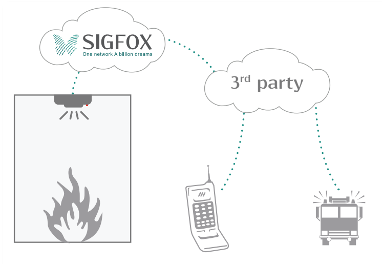
Figure 4. Fire detector solution
