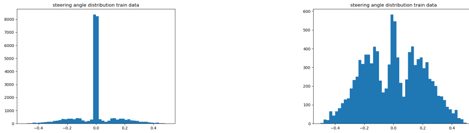
(a) Steering angle histogram before balancing. (b) Steering angle histogram after balancing.
