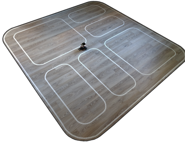
Figure 3.1: The testing and training data collection environment for the jetbot.
