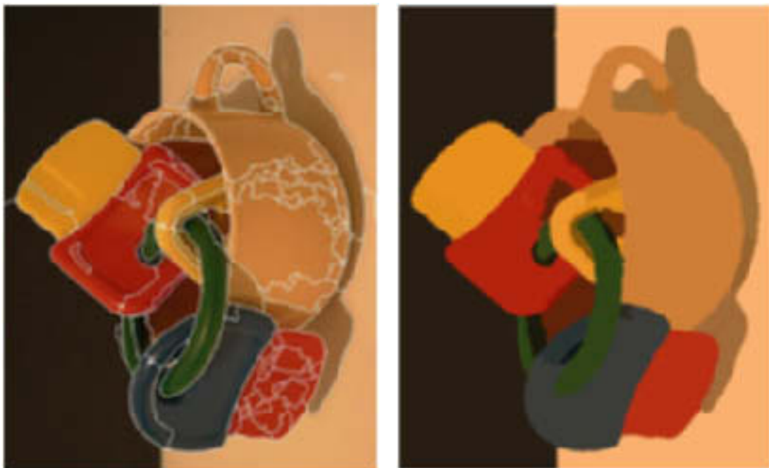
Figure 7.17: The left image shows the result of over-segmenting the image in Fig. 7.16. The right image shows the result of the robust region-merging on the left image after 160 steps. A color version of the two images is presented in Fig.1.3 on page 7.
