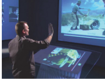
Figure 1. g-speak includes sensor gloves for gesture recognition
