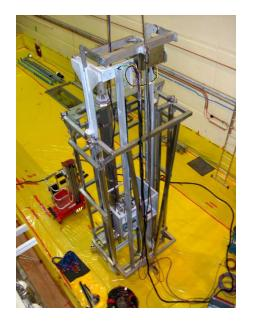
Westinghouse has designed and manufactured a fuel inspection and repair equipment (FIRE)
