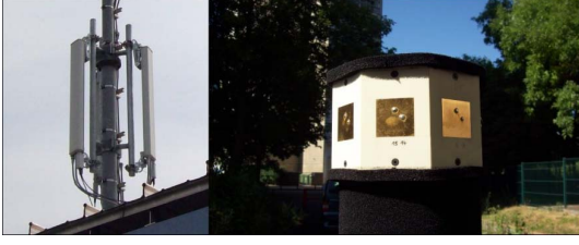
Figure 2. Transmit antenna (left) and receive antenna (right)
