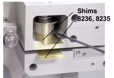
Using Shims for Reassembly
