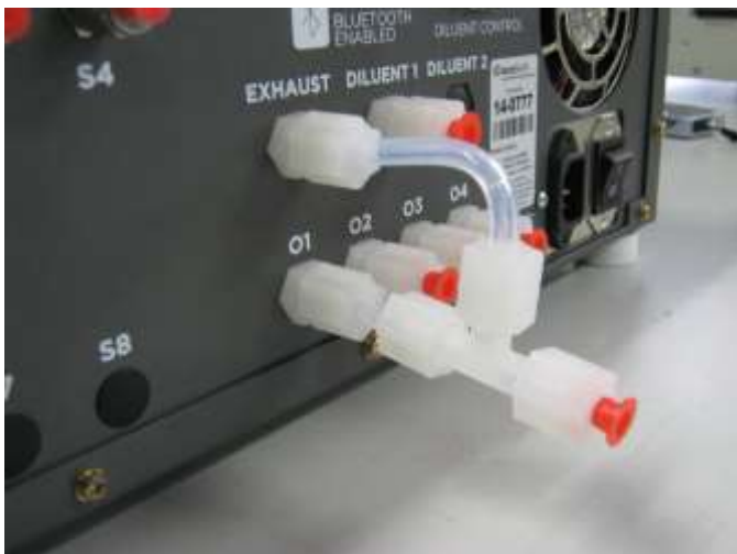
Figure 17 – Connecting the Output and Exhaust Ports Serinus Cal 3000 Only
