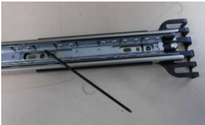
Figure 100 – Attach Rack Mount Adaptors to Outer Slides
