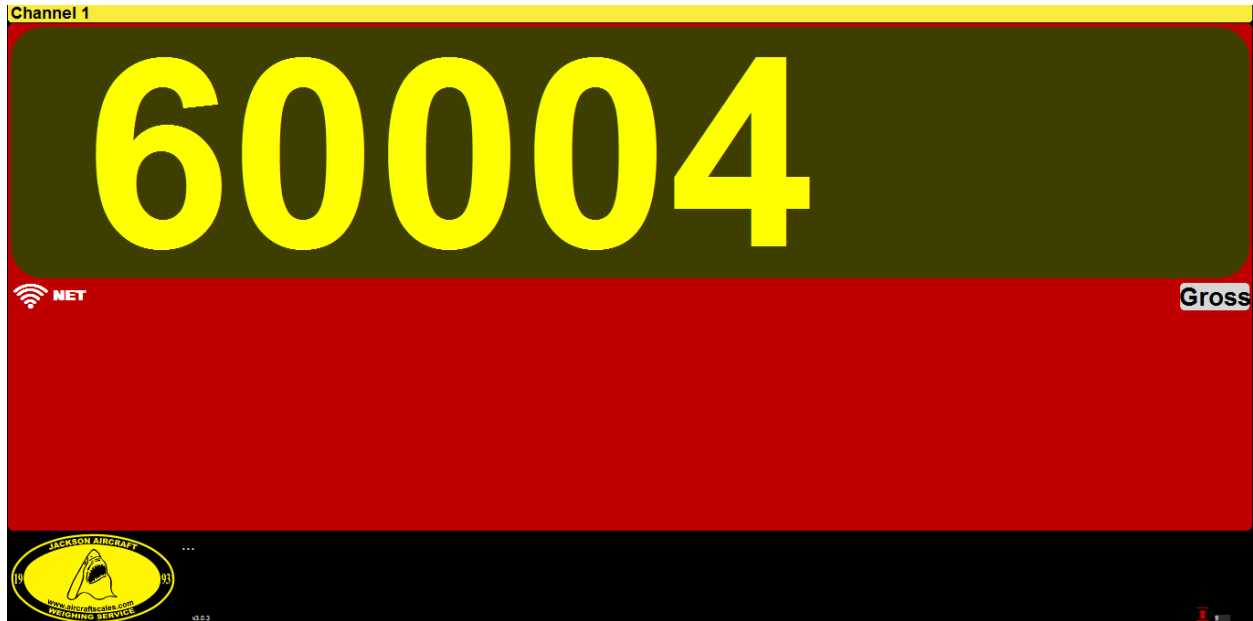
Screen Grab from JAWS software showing a reading of 60,004 with 60,000 lbf applied
